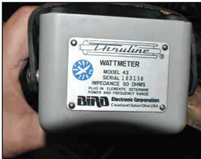
Photo F. Top plate of the Bird Model 43 wattmeter, a very fine test instrument.
