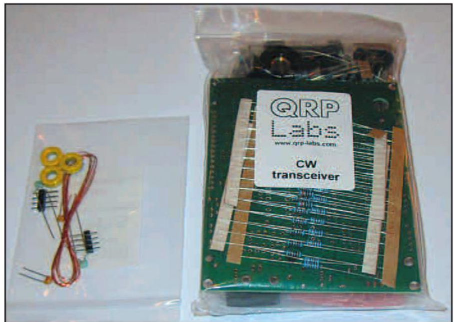
Photo A. The "parts bags" for the QCX transceiver kit. The bigger bag on the right contains components common to all units; the smaller bag on the left holds parts determined by which operating band you choose. (Photos courtesy of the author)
