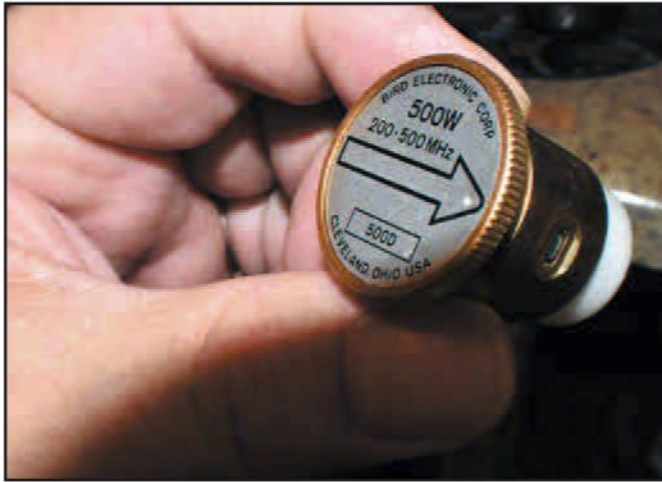
Photo I. Close-up of a Bird slug. The arrow indicates either forward or reflected power, depending on its position within the meter housing. The white area at the bottom of the slug houses the sensing loop.
