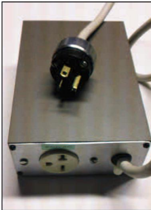
Photo B. Back panel of the soft-start box, showing both the receptacle and plug used in the project.
