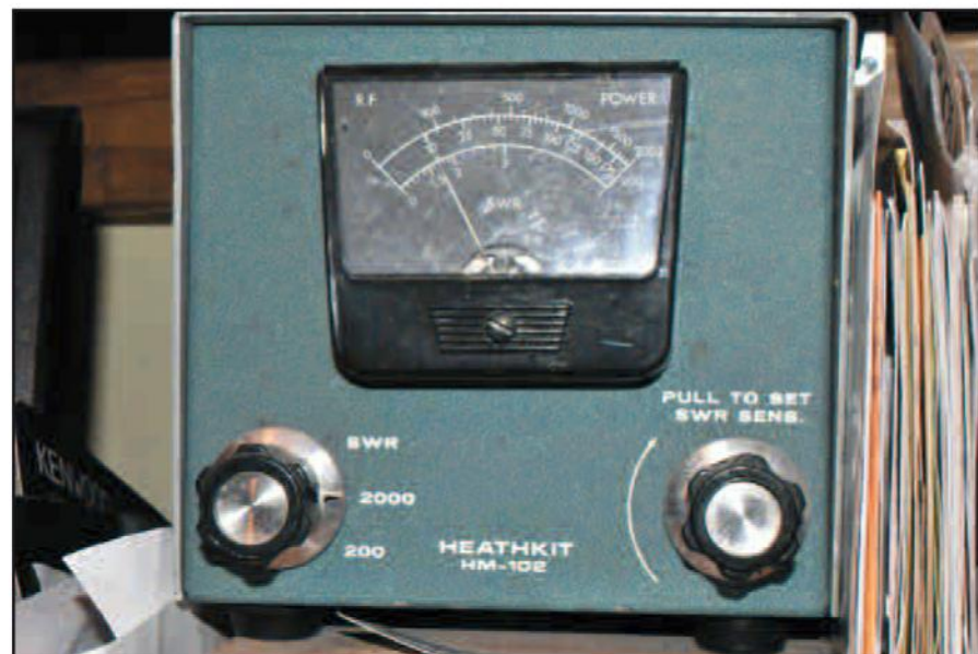
Photo N. Heathkit HM 102 indicating about 75 watts out on HF. This meter is no longer available new, but can be found at hamfests and on the internet.
