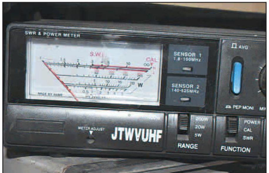
Photo K. Jetstream JTWVUHF meter. HF through UHF in a single meter combination.
