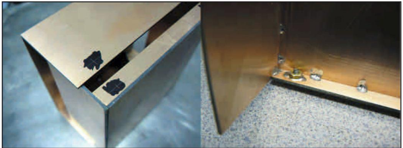
Photo J. Carefully measure and scribe the locations of your screw holes. Once again, measure twice and cut once to ensure that everything will line up properly.
