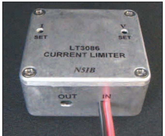
Photo A. Completed current limiter in the suggested die-cast enclosure.
