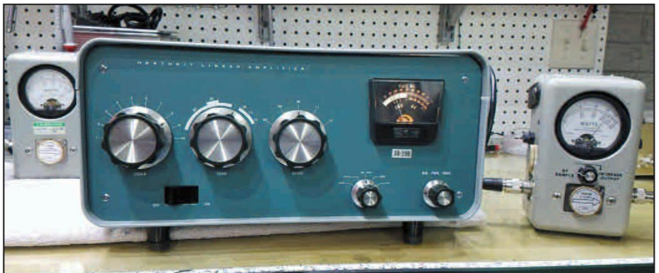
SB-200 hooked to an exciter and dummy load. Eighty watts drive on 20 meters gives 700 watts output.
