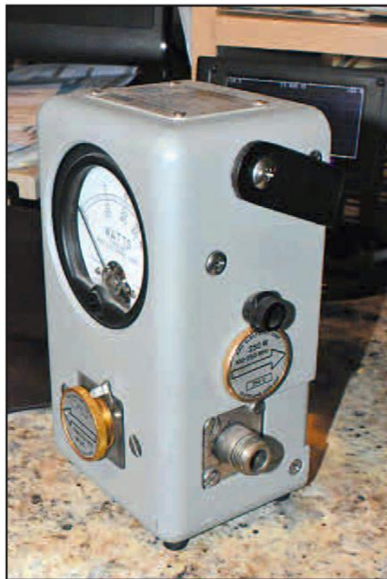
Photo B. The Bird model 43 wattmeter operates on HF, VHF or UHF frequencies, depending on the "slug" that's used. The "N" connectors have better accuracy and lower loss at VHF and UHF.
