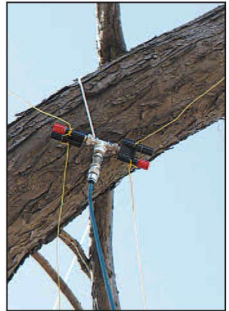
Photo F. Detail of the antenna feed-point. See text for description.
