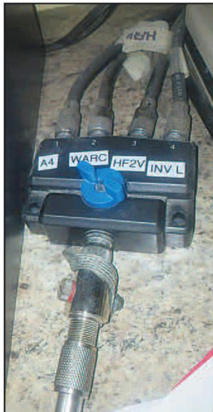
Photo C. A good coax switch allows multiple antennas to be connected to a single transceiver ... and a single wattmeter.
