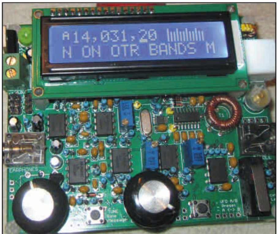
Photo D. The completed QCY transceiver, powered up, on the air and decoding a received CW signal.
