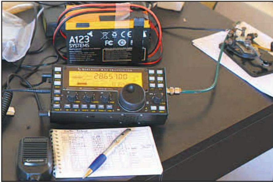
Photo E. CEØY/NCØB ... the QRP station featured an Elecraft KX-3 transceiver, a rechargeable battery and an old J-38 hand key. The author made 25 QSOs during his brief operating periods, the farthest away being Alaska.
