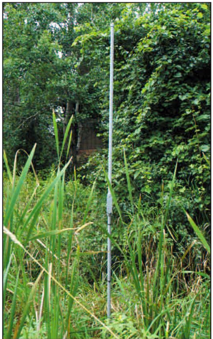
Photo F. The detector and antenna are mounted remotely in the PVC conduit, approximately 120 feet from the transmitting antenna. The length of the connecting twisted pair cable is not critical as long as RF bypassing is addressed properly by C5.
