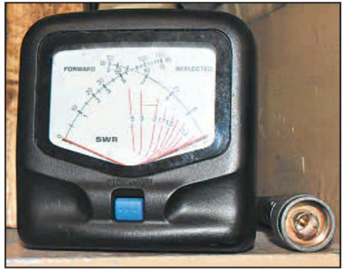
Photo J. Jetstream VHF/UHF meter will indicate power output and SWR at the same time.
