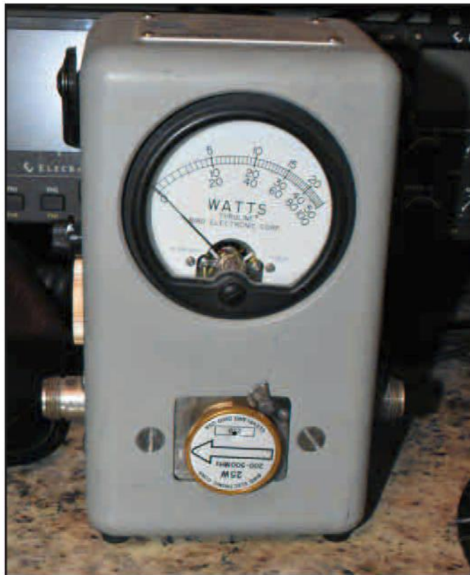
Photo G. A Bird Model 43 wattmeter. Notice the 25-watt, 200- to 500-MHz slug in the front of the meter.
