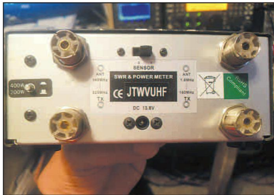
Photo E. Rear panel of the JTWVUHF meter. Notice the VHF/UHF SO-239 connectors for the antenna and transmitter on the left. The HF through VHF connectors are on the right. The selector switch connects the meter circuitry to either port. Note the pushbutton switch for higher power readings of up to 400 watts.
