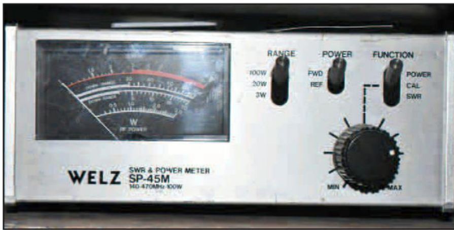
Photo L. Welz SP45 M SWR/wattmeter covers VHF-UHF.
