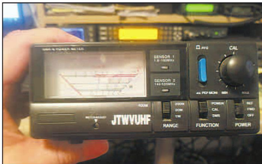
Photo D. The Jetstream JTWVUHF SWR/wattmeter covers HF through UHF. Note the various power settings.
