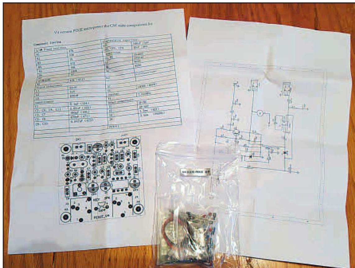
Photo A. The Qianson Pixie Kit...bag of parts, schematic, and parts layout diagram.
