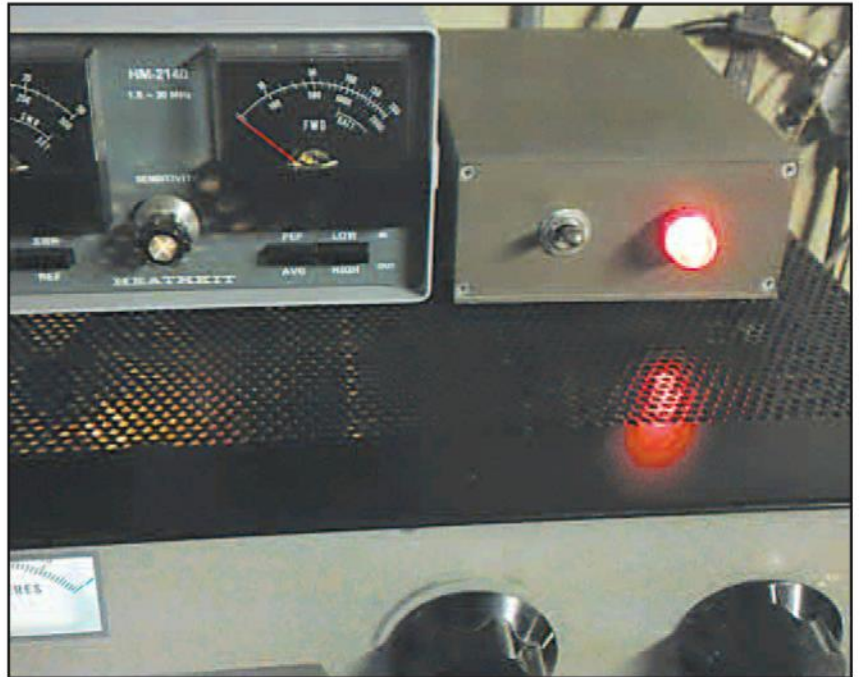
Photo C. The soft-start in use in the author's shack, atop his Drake L4 amplifier. Remember: Turn on the amplifier's power switch first, followed by the soft-start switch.
