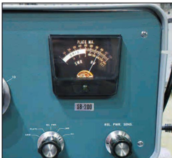
A steady 2,300 VDC is measured on the plates of the output tubes.
