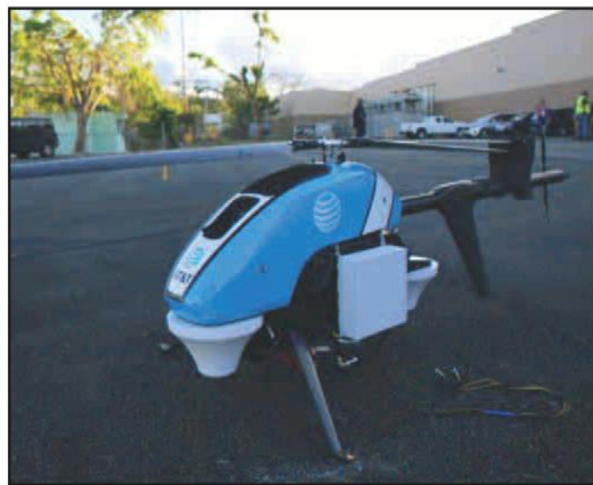
Photo A. Vanu Pulse Vapor 55 drone, outfitted with AT&T LTE cellsite equipment, serves as a “flying COW” or “Cell site on Wings.” (AT&T photo)
