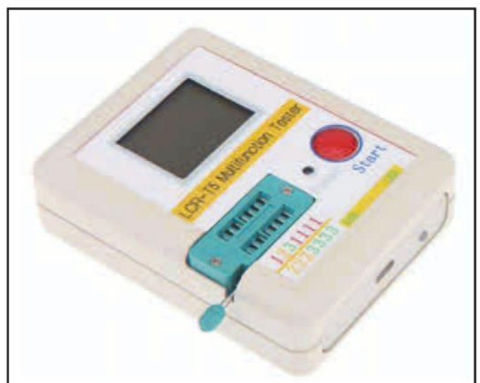
Photo B. A separate component tester, available online in the $20-$30 range, is immensely helpful in identifying component values, especially if the printed codes are too tiny to decipher.
