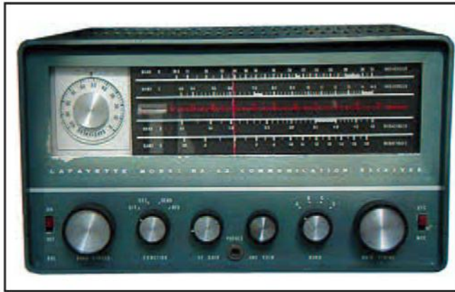
Photo C. My first receiver, a Lafayette HA-63. It used a "band-spread" to tune the 40-meter novice band.
