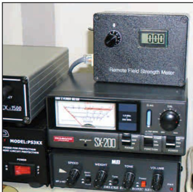
Photo G. The remote readout shows how easy it is to access the field strength reading at the operator's position. →
