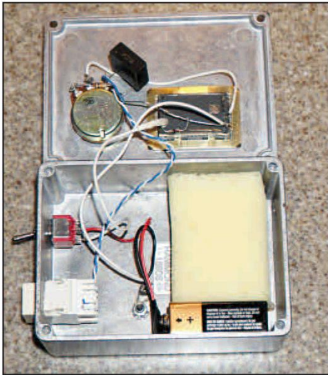
Photo E. The completed remote readout. Note the use of existing terminals on the display and pot to make connections. The 9-volt battery is held snugly using a piece of foam.
