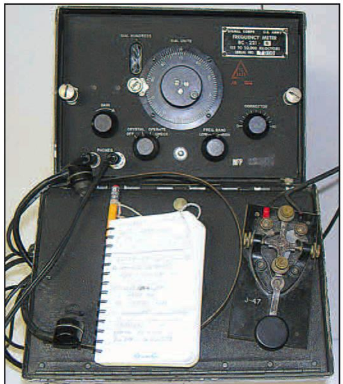
Photo A. The author converted a BC-221 frequency meter — a military staple during World War II — into a 10-watt transceiver for 40 meters. (Photos by the author)
