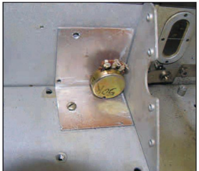
Photo D. A new tuning pot replaced the old (and unusable) gear-drive tuner, but the author needed to make a right-angle bracket in order to mount it at the appropriate spot on the front panel.
