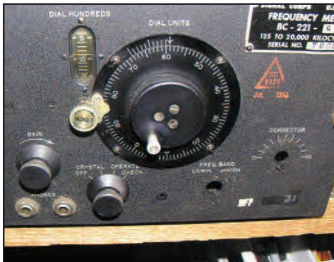
Photo A. The author converted a BC-221 frequency meter — a military staple during World War II — into a 10-watt transceiver for 40 meters. (Photos by the author)
