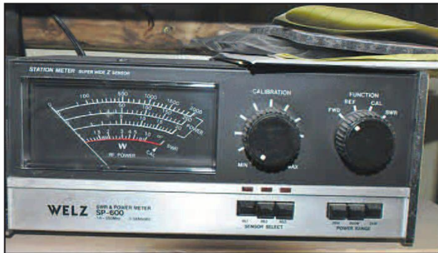
Photo M. Welz SP 600 covers 1.8 to 500 MHz, which makes it very versatile in the shack.
