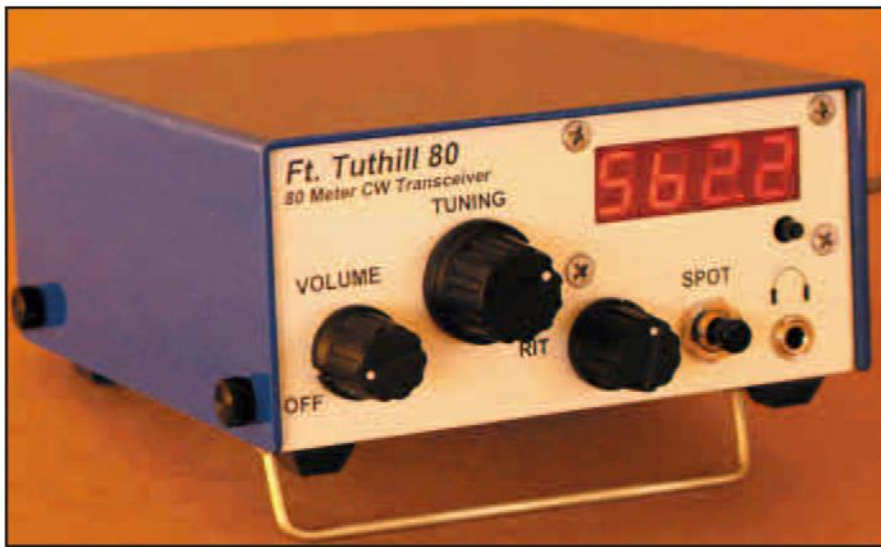
Photo A. The author used copper-clad printed circuit board to build a custom enclosure for his Ft. Tuthill 80 QRP transceiver. The steps shown in this article are specific to this project but may be adapted to your needs.
