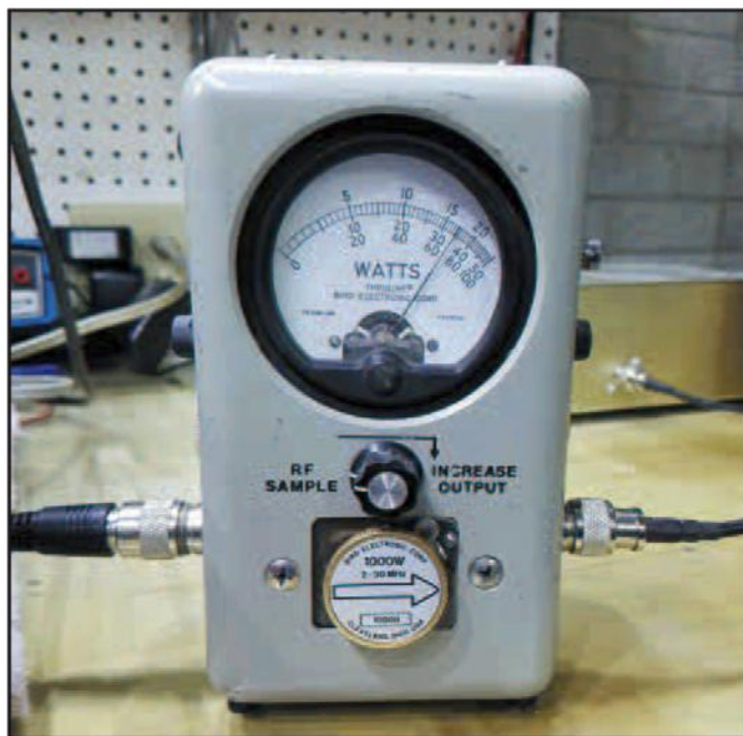
Closeup of Bird wattmeter monitoring power output measured at 700 watts.
